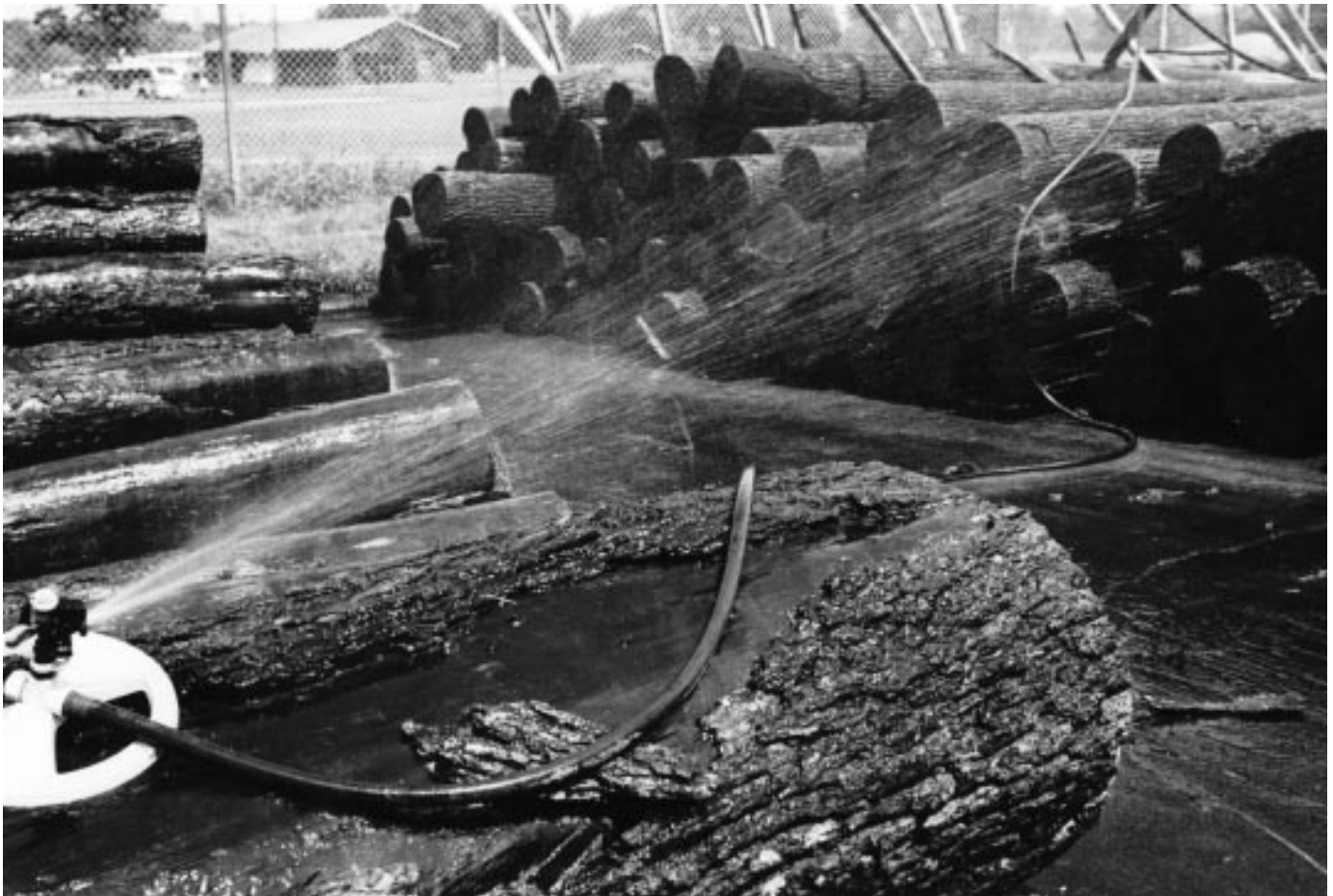
Figure 13-7. Spraying logs with water protects them against fungal stain and decay.
