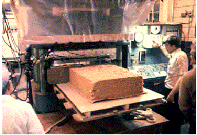
Figure 10–11. Air-laid mat about to enter a laboratory press.
