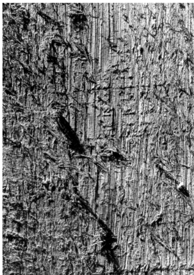
Figure 4-7. Projecting tension wood fibers on sawn surface of mahogany board.
