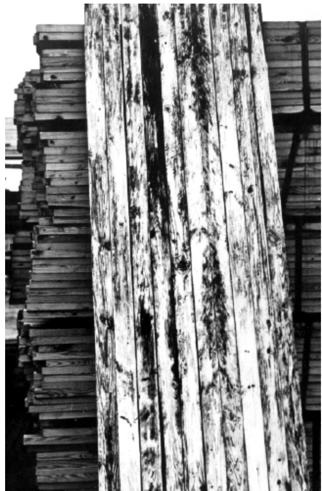
Figure 12-16. Sap stain in Southern Pine. Color ranges from bluish gray to black.
