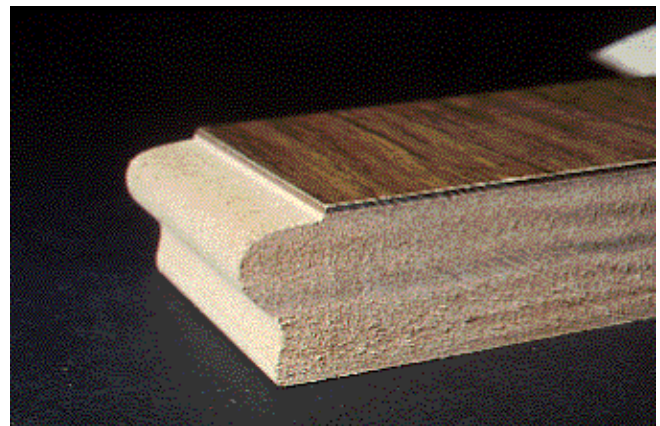
Figure 10–14. Medium-density fiberboard with veneer overlay. Edges can be shaped and finished as required by end product.
